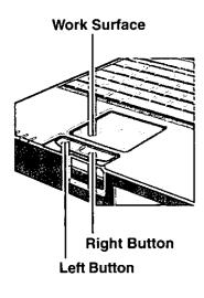
Use the touch pad to move the cursor on the display and perform normal computer operations. For instructions on how to operate, refer to Reference "Touch Pad (Advanced)".
